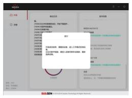
After upgrade is completed, unplug the USB cable, and restart gimbal. Calibrate the Gyro and Acce before the using the gimbal. The current version of the firmware is 01.00.00. Check the gimbal's version of firmware by selecting the 'About' option in the menu.
