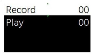
Instructions on How to Operation: Enter the menu, select 'Advanced> 'iFocus'> 'F1'> 'Guidance', then select 'Record' and click the right button. The gimbal will start recording the movement of the smart wheel, recording time is limited one minute. Click the right button on the dial to stop recording. After the recording is completed, select 'Play', and then click the right button on the dial to repeat the recorded motion.
